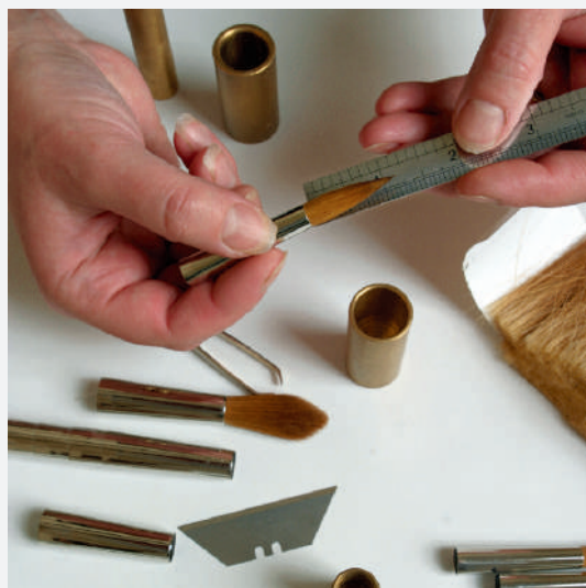
4 Final inspection and measure to check correct 'length out'.
